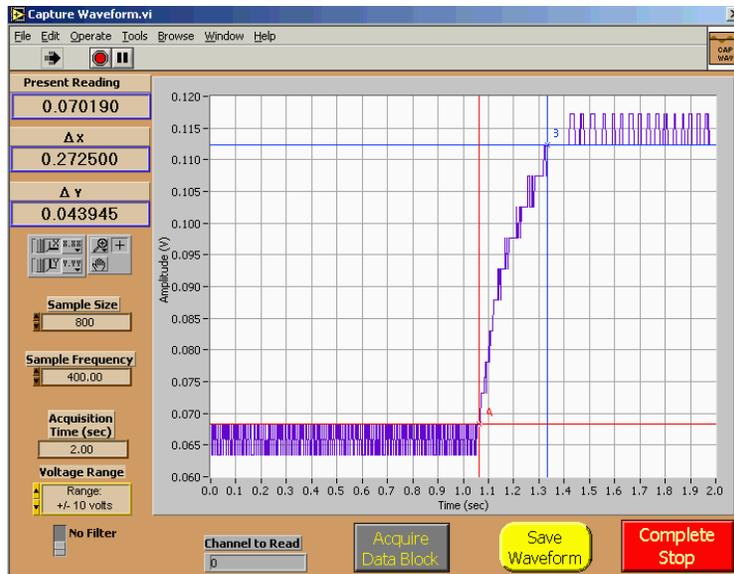
Figure 4. Example thermocouple response curve captured by LabVIEW
