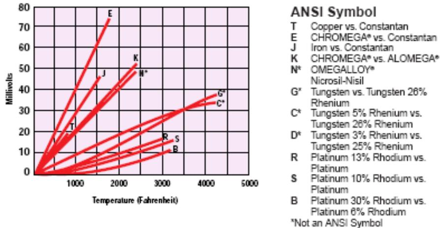
Figure 1. Various thermocouples' response (in voltage) as a function of temperature; of note, a Type-K thermocouple contains alumel (94% nickel, 3% manganese, 2% aluminum, 1% silicon) as the positive (+) electrode and chromel (90% nickel, 10% chromium) as the negative (-) electrode.
