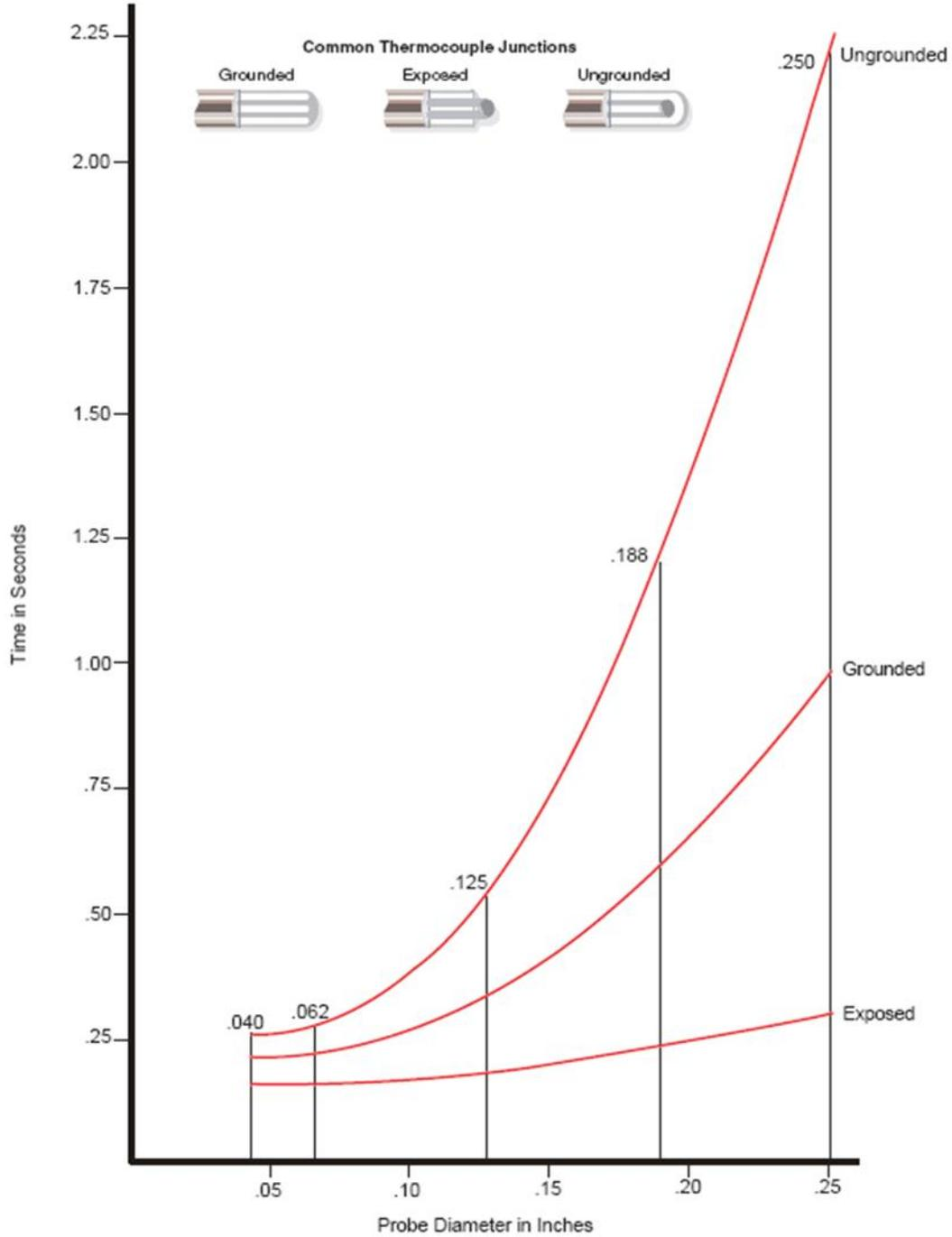
Figure 5. Metal Sheathed Thermocouple Probe Time Response Study in Water
